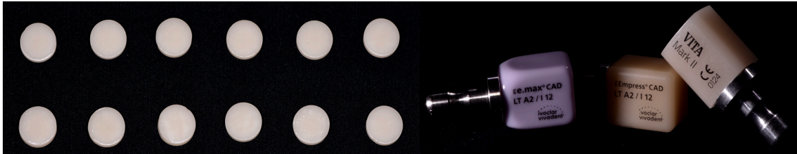
Figure 1: Disc-shaped samples (10-mm diameter and 2-mm thick) of each type of CAD/CAM Monolithic Ceramic
