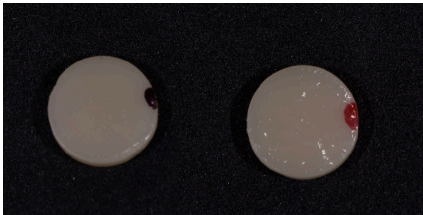
Figure 4:Black and red dots to differentiate between the top and the bottom sides
