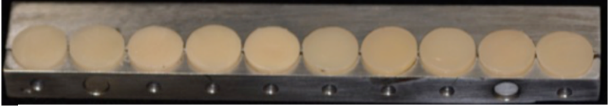
Figure 7: Monolithic ceramic specimens placed in a 10mmx2mm split mold
